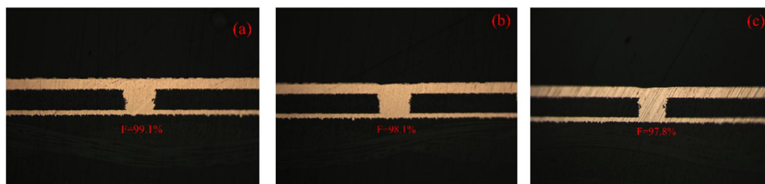
Figure 5. (a), (b), and (c) are cross-sections of the blind holes for each of the three plating experiments.
