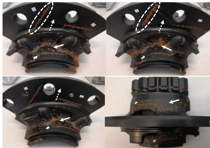
Figure 14. The appearance of the sample coupons after six weeks of accelerated corrosion test, where the solid and broken lines represent the unmachined and machined surfaces, respectively, and broken circles indicate the scribed lines.
