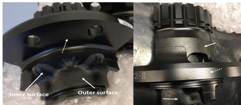
Figure 13. The appearance of the corrosion coupons before the test, where the solid and broken lines represent the unmachined and machined surfaces, respectively.
